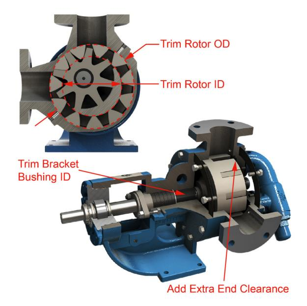
In **high temperature** applications, the extra clearances are needed to allow for expansion of the materials. As a manufacturer, calculations for the clearances are controlled by material selections and are determined based upon a specific material combination within the pump. Changing the part's materials could change the amount of extra clearances needed for the pump.
