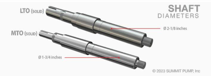
Of course, this also affects the bearing sizes, both inboard (radial) and outboard (thrust), coupling hub size, and consequently the stuffing box size. **The larger shaft diameter directly correlates to a lower Shaft Deflection Index**  $(L^3/D^4)$  rating as well. The lower the number, the less likely the shaft will deflect. See below chart:
