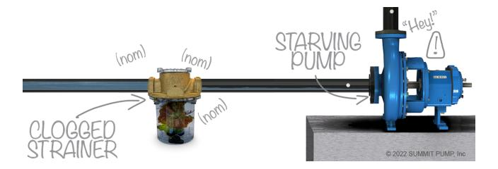
The second issue is that before the strainer fully clogs there is a marked reduction in net positive suction head available (NPSH<sub>A</sub>) causing cavitation. There are also issues with the increase in turbulent flow, because impellers work better if the flow is laminar.
