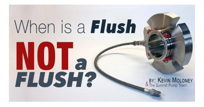
We have all heard the term **"flush"** used when discussing mechanical seals. The definition of a flush is "a stream brought in from an external source to the mechanical seal." This plan (API Plan 32) is almost always used in conjunction with a close clearance throat bushing. The flush fluid must be brought into the stuffing box at a minimum of 15 PSIG higher than stuffing box pressure.
