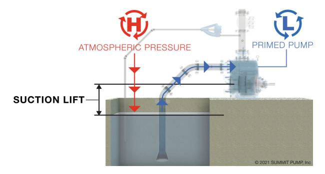
A centrifugal pump cannot "suck" or 'lift" the liquid into itself. Atmospheric pressure is the force pushing the liquid into the pump for open systems. From this information we can conclude; the maximum suction lift at sea level with a perfect pump, a perfect liquid and a frictionless leak free system can approach 34 feet (Atmospheric pressure at sea level is  $14.7 \text{ psia } \text{X } 2.31 \approx 34$ ).
