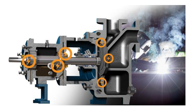
Don't forget that VFD drives are notorious for inducing stray currents into the motor that can travel to the pump and create bearing damage. Make sure the equipment is grounded.
