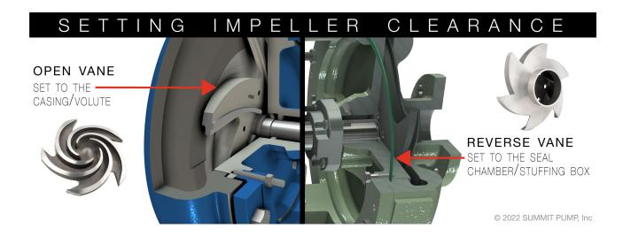
In general, the reverse vane impeller clearance is established to the stuffing box and the open impeller style is matched to the casing. Each design has its pros and cons. Considering all the possible pump application variables neither style is the overall winner. The requirements of each application should dictate the design choice.
