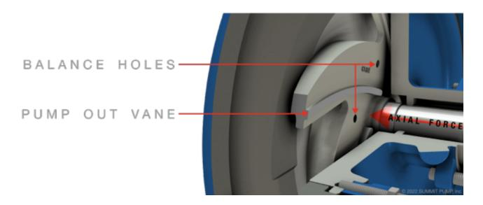
Do not use impellers with balance holes in lift situations as the potential for liquid product flashing in the seal chamber increases.
