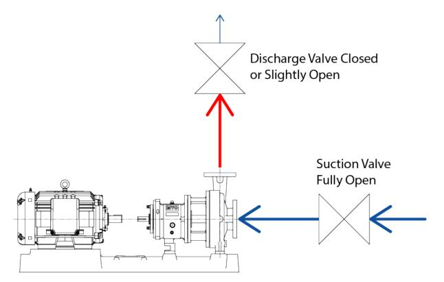
In case of higher pressure applications, it would be difficult or almost impossible to manually operate the valve if it was fully closed. The closer you get to an axial flow pump, with higher specific speeds, the more important it is to have the valve wide open. This is because the pump requires maximum horsepower at low flow. The horsepower requirements drop as the flow approaches BEP and right side of the pump curve.
