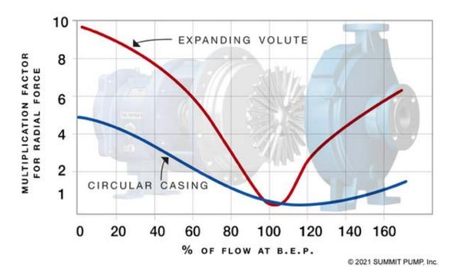
Low flow pumps utilize a *circular casing* where the casing is concentric to the impeller. By utilizing this design the radial thrust component can be appreciably reduced by amounts, normally in the range of 65 to 85%. In many cases using a low flow pump will reduce the need and cost for the more robust shaft (lower L over D ratio) and bearing system.
