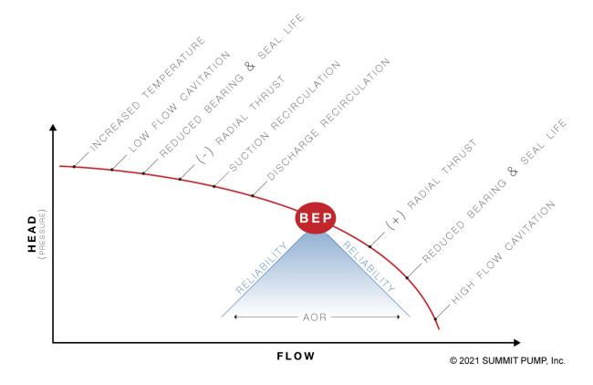
Of course, most end users don't have just one operating point and normally they want to operate in a wide area that is commonly referred to as a safe or allowable operating region (AOR). Therefore, most pump applications will require operation away from the area of BEP.
