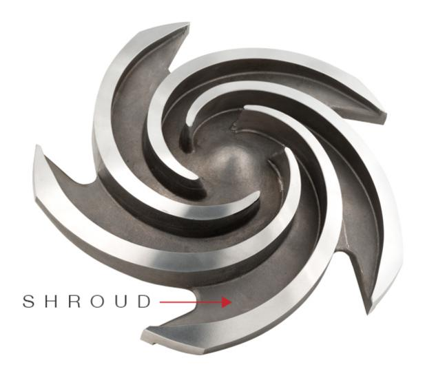
ANSI style (B73.1) pumps are end suction types that use semi open impellers 99% of the time. These impellers have a **shroud** on one side only. This geometry makes them easy and less expensive to manufacture. However, a downside consequence is an impeller with higher unbalanced axial forces.
