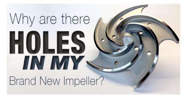
Ever wonder why some impellers, fresh and new from the factory have holes in them? Or... why some impellers have those funny mini vanes on the back side? The short answer is to reduce the axial thrust in the pump and also to reduce the pressure in the stuffing box.
