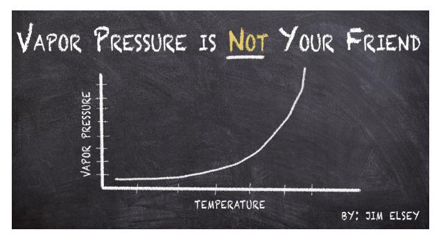
Be very careful on self-primer lift applications because the liquid temperature directly affects its vapor pressure and that...
