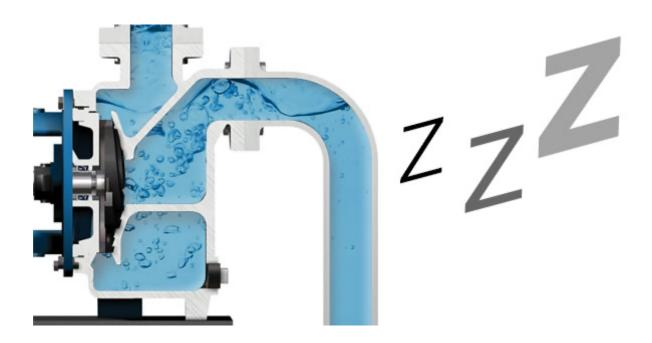
Snoring is usually a term reserved for submersible pumps on dewatering applications at construction sites, but the phenomena can apply to most any centrifugal pump type and application.
