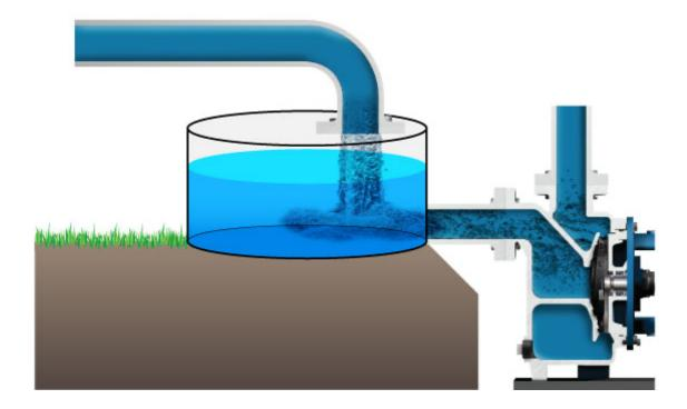
One of the main culprits for pump snoring is simply poor sump design, where the influent is dumped into the sump at elevations high above the liquid level at or near the pump suction intake without the benefit of weirs or baffles. This improper geometrical arrangement contributes to a "waterfall effect" pulling air into the liquid...it probably should be called the "water torture" method.
