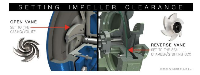
Both impeller designs have their pros and cons. For example, the reverse vane impeller can be accurately set without the casing in the safe and controlled environment of a shop. The open impeller design normally offers a larger wear area that may translate to longer periods of reliable and less costly operation. The reverse vane impeller presents a consistent lower seal chamber pressure (note: check for vapor pressure issues). The open impeller handles stringy and fibrous solids better.
