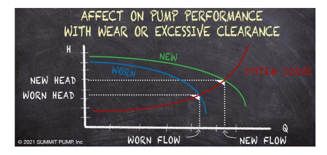
The general "rule of thumb" is that the pump will lose about 1% of its capacity for each 0.001 inches of impeller clearance for the first 0.005 to 0.008 inches of added clearance over the initial setting. The issue gets markedly worse with increasing clearance.
