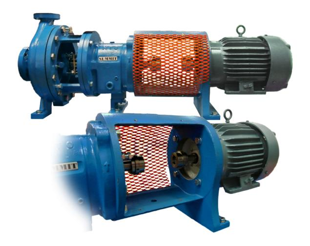
When using *best industry practices* you need less than 0.002" for pump/motor alignment, not the 0.007" to 0.015" T.I.R. The good news is that the C-Face adapter will hold the published alignment. Traditional arrangements, if improperly installed base plate, foundation, piping and piping design can quickly cause large shaft misalignment.
